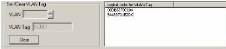
In addition to the VLAN provisioning box, a second box appears to the right that is used to display a list of all logical links in the provisioned VLAN. No links will be displayed in this box until the VLAN provisioning is applied. Clicking on a logical link in this list allows the user to quickly change the context of the panel to the other logical link. This is useful when changing links to a different VLAN.
