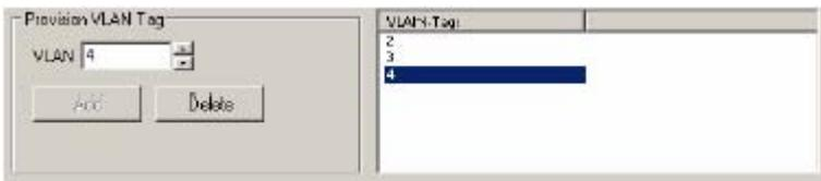
A box to the right of the provisioning window is used to display all of the VIDs associated with a particular logical link provisioned in Transparent VLAN. Selecting a VID in the box moves it into the provisioning window, allowing it to be quickly deleted. Once a VID is deleted the VLAN field in the provisioning window will take on one of the other provisioned values, allowing all VLANs to be quickly deleted with repetitive mouse clicks.
