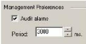
**Step 3.** By default the GUI does not display the reports generated by alarm audits. To enable the GUI to display alarm audits in the GUI Log Window, check the box labeled “Log all alarm audits.”
