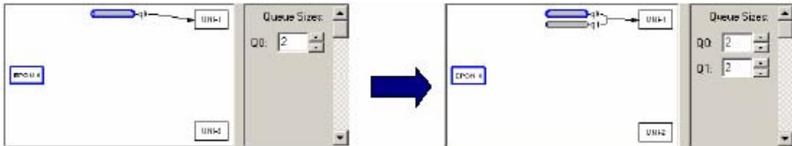
**Step 2.** Use the Num Qs control to add a second FIFO, by changing the value from 1 to 2. Notice that a second FIFO will appear in the diagram as depicted in the figure above.
