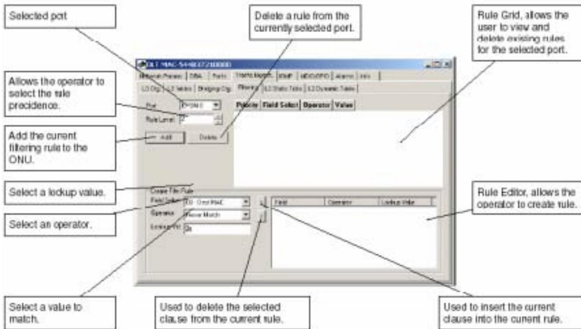
This panel allows the operator to create rules to filter (drop received frames), based on many different criteria (Rules).
