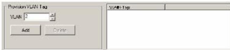
The “Add” button is used to add a VID and the “Delete” button is used to remove a VID.
