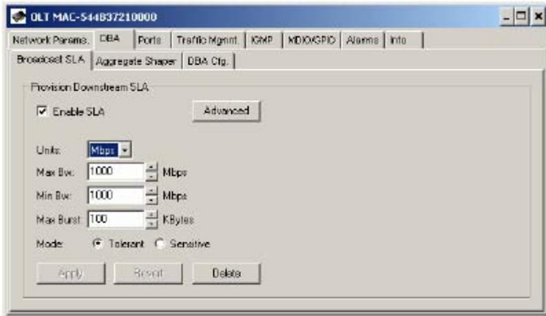
This command is identical to the functionality of the Link SLA Panel except that it is used to provision an SLA for the broadcast channel, as apposed to a unicast link. This unique feature of the OLT allows the OLT To use its large 40Meg buffer ram to serve the requirements of all ONUs, resulting in a 1:32 cost reduction (assuming 32 ONU deployment).
