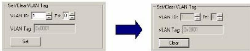
Notice that after the VLAN has been provisioned the panel will change to a grey color. The user must delete the VLAN provisioning before applying a new tag value. Once a VLAN has been provisioned, the OLT will not permit the bridging mode to be changed without first deleting the VLAN provisioning. If an attempt is made to change the bridging mode, the GUI will display a dialog box allowing the user an opportunity to automatically delete the VLAN provisioning.
