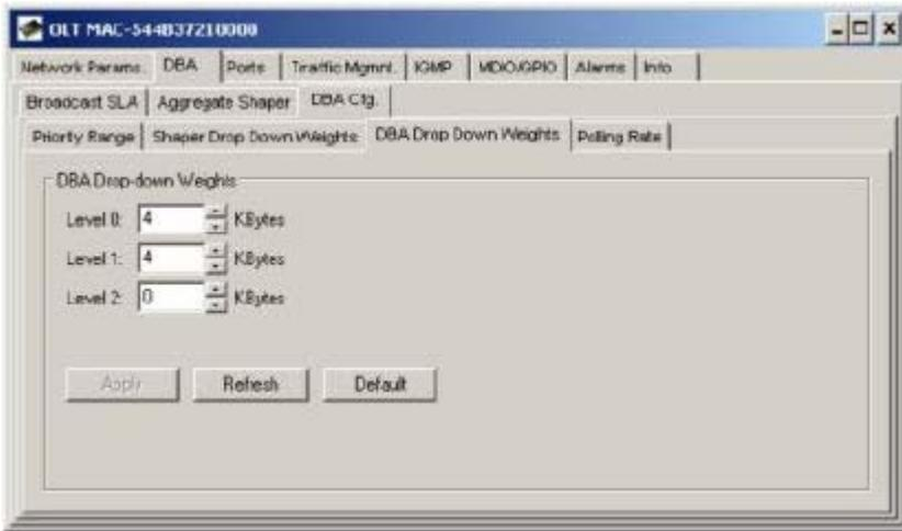
DBA drop down weights are used by the DBA to reserve bandwidth for each priority level. This allows the OLT to fix the latency and reserve a percentage of bandwidth for links in each priority level. The drop down weight for priority level  $n$  **MUST** be greater than or equal to the provisioned DBA Weight for all links in priority level  $n + 1$ .
