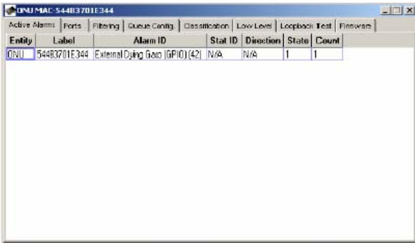
The GUI Alarm Log will display a new entry, retained until the GUI is terminated. The GUI Alarm Log will indicate the way in which a particular alarm was detected, or the reason why it was cleared in the column labeled Disposition. The GUI has 3 different alarm “dispositions”: autonomous, audit, and internal.
