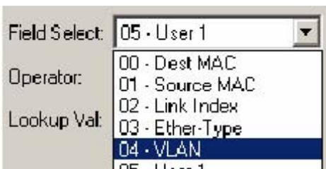
**Step 2.** Choose an appropriate Operator. The operator tests the portion of the frame specified by the field select.
