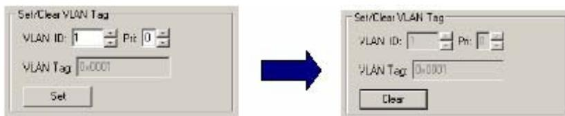
Once a value has been entered for VLAN ID and Pri (CoS), the “Set” button may be used to apply the provisioning. The “Clear” button is used to delete the provisioned tag.
